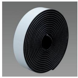
$3M^{\text{TM}}$  Dual Lock<sup>TM</sup> Reclosable Fastener SJ3541 has a rubber based adhesive on the back of a black, polypropylene reclosable fastner.  $3M^{\text{TM}}$  Dual Lock<sup>TM</sup> Reclosable Fastener SJ3540 has a 400 stems per square inch with a 0.23 inch engaged thickness. The closure life is 1,000 times.
