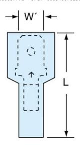
This terminal has a wire range of 16-14 AWG and has case quantities of 1000 per case.
