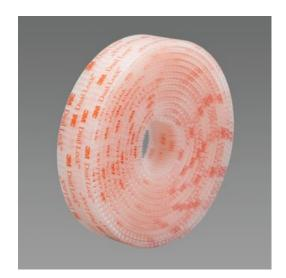
3M™ Dual Lock™ Reclosable Fastener SJ3560 has a clear acrylic adhesive on the back of a clear polypropylene reclosable fastener with 250 stems per square inch and 0.23 inch engaged thickness. 3M™ Dual Lock™ Reclosable Fastener SJ3560 has a closure life of 1,000 times.
