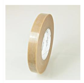
This .0055 inch thick tape is a polyester web reinforced polyester film coated with a rubber pressure-sensitive adhesive. On a 3 inch paper core this puncture-resistant tape is tough and conformable with excellent electrical properties.
