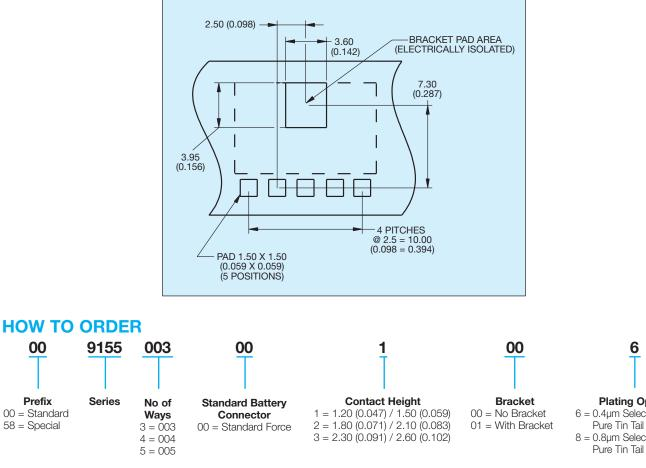
**Plating Option** 6 = 0.4µm Selective Gold, Pure Tin Tail 8 = 0.8µm Selective Gold,
