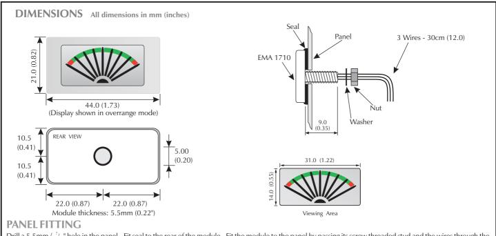
Drill a  $5.5 \, \text{mm} / \, \, ^7 \! / _{32} \, ^{\text{\tiny II}}$  hole in the panel. Fit seal to the rear of the module. Fit the module to the panel by passing its screw threaded stud and the wires through the hole, fitting the washer and tightening the nut. Take care not to trap any of the connecting wires. Do not to overtighten the nut as this may damage the meter.
