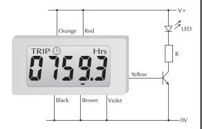
Using the PULSE O/P to drive an LED. The LED will illuminate once after every hour.
