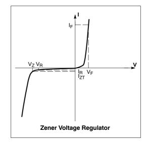
**ELECTRICAL CHARACTERISTICS** ( $T_A = 25^{\circ}C$  unless otherwise noted,  $V_F = 1.2$  V Max @  $I_F = 1.0$  A for all types)
