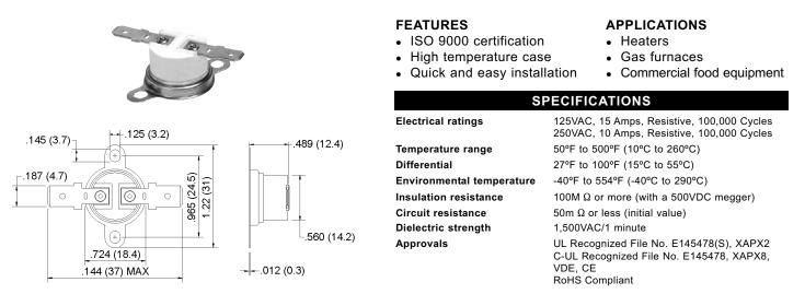
These snap-action bimetal discs are housed in a ceramic case to handle extremely high temperatures. The increased factory calibrated set points are available up to 500°F (260°C). The contacts can either open or close on temperature rise.
