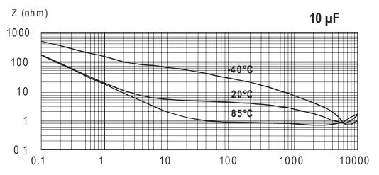
R<sub>e</sub> is the most temperature-dependent component of an electrolytic capacitor equivalent circuit. Electrolyte resistivity will decrease if temperature rises.
