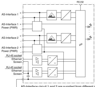
AS-Interface circuit 1 and 2 are supplied from different power supplies. At the cable for power supply no slaves or repeaters may be attached. At the cable for AS-Interface circuit no power supplies or further masters may be attached.
