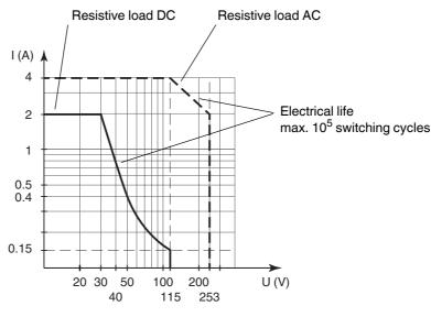
The maximum number of switching cycles is depending on the electrical load and may be higher when reduced currents and voltages are applied.
