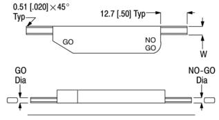
Inspection of Wire Crimping Chamber
