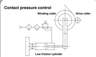
Adapts to the cylinder's piston displacement, maintaining a constant pressure.
