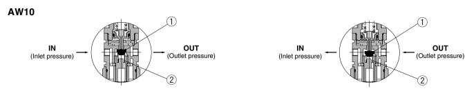
When the inlet pressure is higher than the regulating pressure, the check valve operates as a normal regulator (Figure 1).
