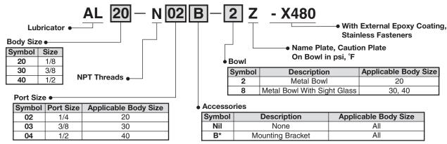
\*Note: Bracket is not assembled and is supplied loose at time of shipment.
