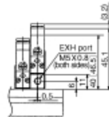
Dimensions when mounting individual EXH spacer
