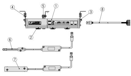
Note 2) For cases where the potential of a charged object is measured using a feedback sensor, the relationship between the potential being measured, the sensor monitor output voltage and the detection range of the sensor will vary depending on the sensor's installation distance. Refer to page 3.
