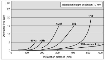
Air purge: Yes Supply pressure: 0.05 MPa (3.5 t/min (ANR) per nozzle)
