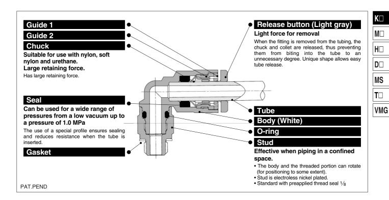
Optimum piping in less space with 20% reduction of the outside diameter
