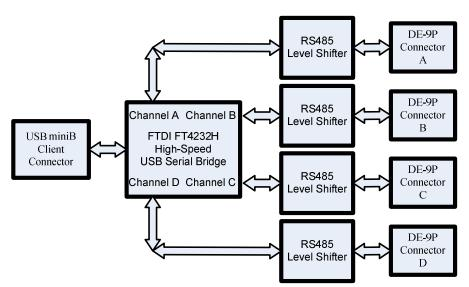
Figure 1.2 USB-COM485-PLUS4 Block Diagram
