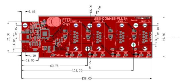
Figure 5.1 - USB-COM485-PLUS4 PCB Dimensions
