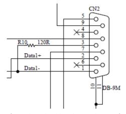
Figure 2.1 USB-COM485-PLUS4 Termination resistor
