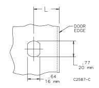
Designed for field installation in standard one-door Type 3R and 12 enclosures. Includes complete installation instructions. One hole must be drilled or punched in the door to receive the cylinder lock.
