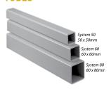
Square and rectangular tubes are cold-formed, hollow, welded steel with 5-mm wall thickness. Finish is RAL 7035 light-gray polyester powder paint
