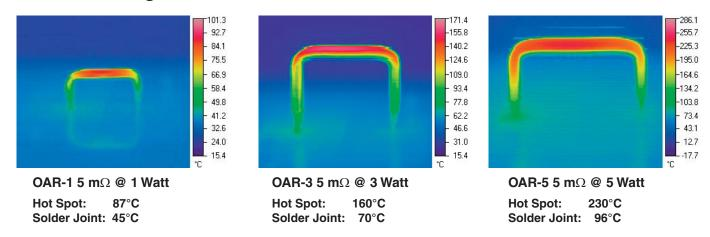
The thermal images (not simulations) above are of the OARs products at their respective power rating. Notice the solder joint temperature is much lower than the hotspot. The unique construction of the OAR isolates the temperature of the hotspot from the circuit board material preventing damage to the circuit board. Additionally, the thermal energy is dissipated to the air instead of being conducted into the circuit board potentially causing a nearby power component to exceed its rating.
