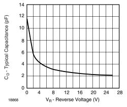
Figure 2. Diode Capacitance vs. Reverse Voltage  $V_{\mathsf{R}}$
