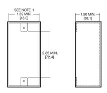
MINIMUM INTERIOR DIMENSIONS FOR INSTALLATION INTO A STANDARD UTILITY BOX
