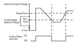
The 120AZ and 240AZ voltage sensors are intended for use as protection devices for electronic equipment in the event of a brown out condition.
