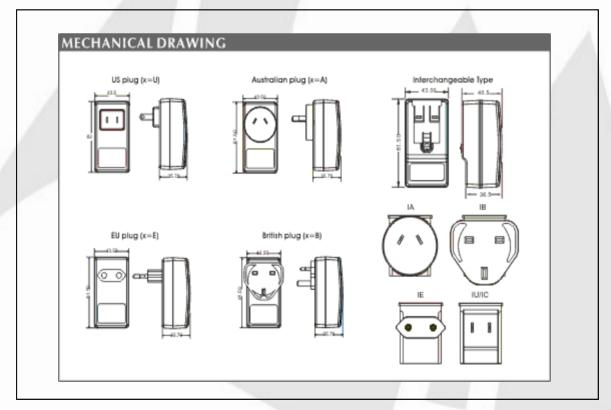
A full set of connectors is delivered with each product order. If a specific connector Is required then add a U,A,E or B to the I suffix on your order.
