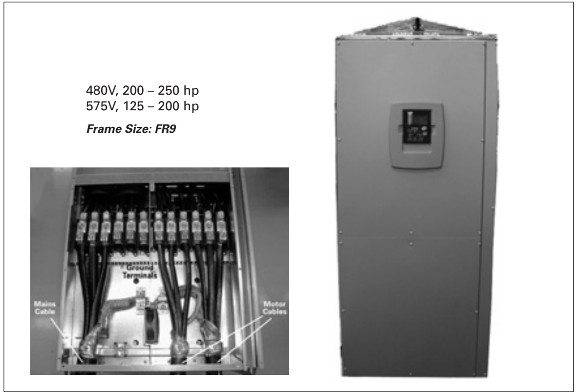
Figure 3-13: FR9 Power and Motor Wiring Terminals
