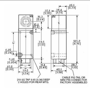
$\, ^{\scriptsize \textcircled{\scriptsize 1}}$  Can accommodate both U.S., 29.4 [1.16] x 59.5 [2.34] and DIN, 30 [1.18] x 60 [2.36], mounting dimensions.
