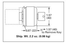
Figure 47-48. E22/EM22 Series 40 mm Dia. Key Release Button
