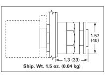
Figure 47-56. E22/EM22 Series 3-Position 40 mm Dia. Lens (Spring Return to Center)
