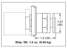
Figure 47-54. E22/EM22 Series 3-Position 40 mm Dia. Push-Pull Pushbutton (Spring Return to Center from Pulled Position)
