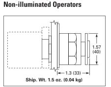
Figure 47-52. E22/EM22 Series 2-Position 40 mm Dia. Button (Maintained)
