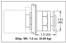
Figure 47-57. E22/EM22 Series 3-Position 40 mm Dia. Push-Pull Pushbutton (Spring Return to Center from Pulled Position)
