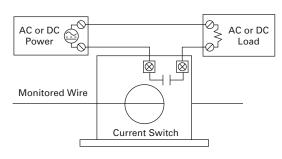
NOTE: The above diagram is for Normally Open (N.O.) models.
