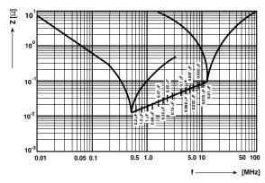
Impedance (Z) as a function of frequency (f) at  $T_a = 20$  °C (average). Measurement with lead length 6 mm.
