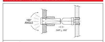
Pass LITEPIPE® through panel opening. Press on retaining ring. Air gap .050" maximum between LED and LITEPIPE® for best performance.
