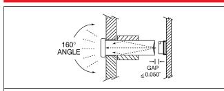
Pass LITEPIPE  $^{\circ}$  through panel opening. Press on retaining ring. Air gap .050  $^{''}$  maximum between LED and LITEPIPE  $^{\circ}$  for best performance.
