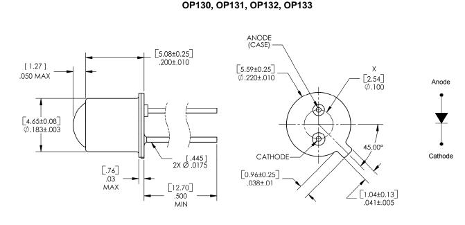
X THIS DIMENSION CONTROLLED AT HOUSING SURFACE.
