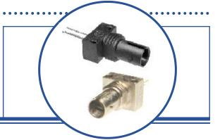
The OPF79X is a low noise silicon PIN photodiode mounted in a low cost package for fiber optic applications. It offers fast response at moderate bias and is compatible with LED and laser diode sources in the 800-1000 nm wavelength region. Low capacitance improves signal to noise performance in typical short haul LAN applications.
