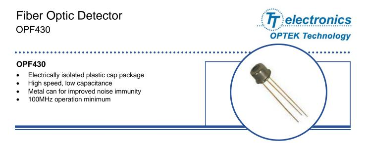
The OPF430 is a low noise silicon PIN photodiode mounted in a low cost package for fiber optic applications. It offers fast response at moderate bias and is compatible with LED and laser diode sources in the 800-1000 nm wavelength region. Low capacitance improves signal to noise performance in typical short haul LAN applications.
