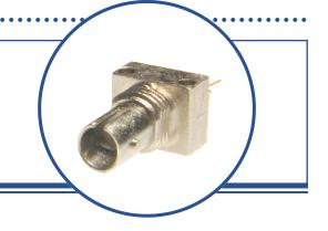
The OPF372 family fiber optic transmitters are high performance devices packaged for data communication links. This transmitter is an 850nm GaAlAs LED and is specifically designed to efficiently launch optical power into fibers ranging in size from 50/125µm up to 200/300µm diameter fiber. Multiple power ranges with upper and lower limits are offered which allows the designer to select a device best suited for the application.
