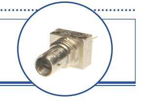
The OPF422 is a low noise silicon PIN photodiode mounted in a low cost package for fiber optic applications. It offers fast response at moderate bias and is compatible with LED and laser diode sources in the 800-1000 nm wavelength region. Low capacitance improves signal to noise performance in typical short haul LAN applications.
