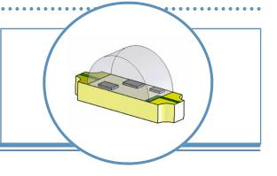
The **OVSRRGBCC3** is a compact full-color (RGB) in a miniature surface mount package with a 150° viewing angle. This 1204 package provides the option to mount it as a top-emitting or side-emitting (right angle) device. The device can be used on smaller boards with a higher packing density and is ideal for handheld applications.
