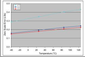
**FIGURE 2-32:** Zero-Scale Error (ZSE) vs. Temperature (MCP4716).  $V_{DD} = 5V, V_{REF1}: V_{REF0} = 10, G = 0,$  $V_{REF} = V_{DD}$ .
