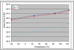
**FIGURE 2-82:** Output Error vs. Temperature (**MCP4726**).  $V_{DD}$  = 2.7V and 5V,  $V_{REF1}$ : $V_{REF0}$  = 10, G = 0,  $V_{REF}$  =  $V_{DD}$ , Code = 4000.
