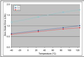
**FIGURE 2-49:** Zero-Scale Error (ZSE) vs. Temperature (**MCP4726**).
