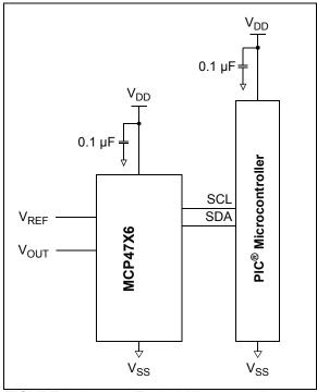
FIGURE 8-10: Typical Microcontroller Connections.
