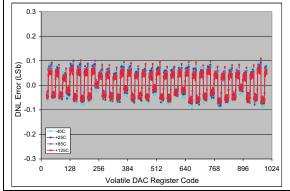
FIGURE 2-8:DNL vs. Code (code = 25 to1000) and Temperature (MCP4716). $V_{DD}$  = 5V,  $V_{REF1}$ :  $V_{REF0}$  = 00.
