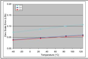
FIGURE 2-33:Zero-Scale Error (ZSE) vs.Temperature (MCP4706). $V_{DD} = 5V$ ,  $V_{REF1}$ :  $V_{REF0} = 10$ , G = 0, $V_{REF} = V_{DD}$ .
