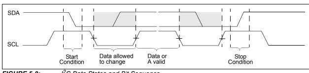
**FIGURE 5-8:** I<sup>2</sup>C Data States and Bit Sequence.
