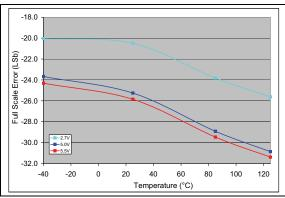
**FIGURE 2-16:** Full-Scale Error (FSE) vs.  $V_{DD}$  and Temperature (**MCP4726**).  $V_{REF1}$ : $V_{REF0} = 00$ .
