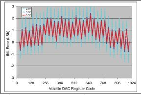
**FIGURE 2-56:** INL vs. Code (code = 25 to 1000) and  $V_{DD}$  (2.7V, 5V, 5.5V) (**MCP4716**).  $V_{REF1}:V_{REF0} = 10, G = 1, V_{REF} = V_{DD}/2,$ Temp = +25°C.
