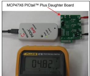
**FIGURE 9-2:** MCP47X6 PICtail Plus Daughter Board with PICkit<sup>™</sup> Serial Analyzer.
