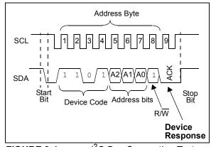
FIGURE 8-1: I<sup>2</sup>C Bus Connection Test.
