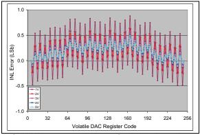
**FIGURE 2-75:** INL vs. Code (code = 6 to 250) and  $V_{REF}$  (MCP4706).  $V_{DD} = 5V$ ,  $V_{REF1}$ : $V_{REF0} = 11$ , G = 0,  $V_{REF} = 1V$ , 2V, 3V, 4V, and 5V, Temp = +25°C.
