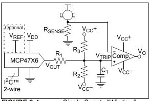
FIGURE 8-4: Single-Supply "Window" DAC.
