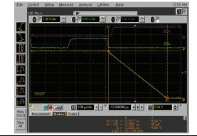
FIGURE 2-97: Full-Scale Settling Time (FFFh to 000h) (MCP4726).
