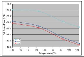
FIGURE 2-34: Full-Scale Error (FSE) vs. Temperature (MCP4726).
