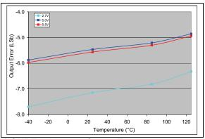
**FIGURE 2-83:** Output Error vs. Temperature (MCP4716).  $V_{DD} = 2.7V$  and 5V,  $V_{REF1}:V_{REF0} = 10$ , G = 0,  $V_{REF} = V_{DD}$ , Code = 1000.
