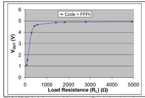
**FIGURE 2-94:**  $V_{OUT}$  vs. Resistive Load.  $V_{DD}$  = 5.0V.
