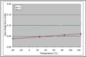
**FIGURE 2-51:** Zero-Scale Error (ZSE) vs. Temperature (**MCP4706**).
