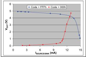
**FIGURE 2-95:**  $V_{OUT}$  vs. Source/Sink Current.  $V_{DD}$  = 5.0V.
