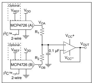
**FIGURE 8-7:** Simple Double Precision DAC using MCP4726.
