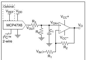
**FIGURE 8-5:** Digitally-Controlled Bipolar Voltage Source Example Circuit.
