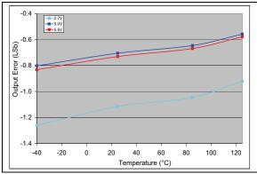
**FIGURE 2-81:** Output Error vs. Temperature (MCP4706).  $V_{DD}$  = 2.7V and 5V,  $V_{REF1}$ :  $V_{REF0}$  = 00, Code = 250.
