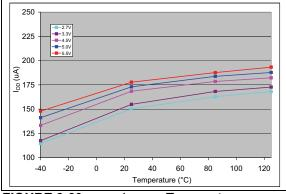
FIGURE 2-89: $I_{DD}$  vs. Temperature. $V_{DD}$  = 2.7V and 5V,  $V_{REF1}$ :  $V_{REF0}$  = 10, G = 0, $V_{REF}$  =  $V_{DD}$ .
