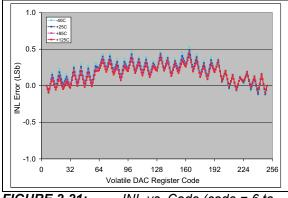
FIGURE 2-21:INL vs. Code (code = 6 to250) and Temperature (MCP4706). $V_{DD} = 5V$ ,  $V_{REF1}$ :  $V_{REF0} = 10$ , G = 0, $V_{REF} = V_{DD}$ .
