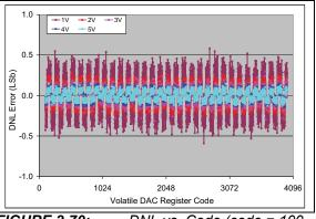
**FIGURE 2-70:** DNL vs. Code (code = 100 to 4000) and  $V_{REF}$  (**MCP4726**).  $V_{DD} = 5V$ ,  $V_{REF1}$ :  $V_{REF0} = 10$ , G = 0,  $V_{RFF} = 1V$ , 2V, 3V, 4V, and 5V, Temp = +25°C.
