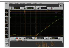
**FIGURE 2-100:** Exiting Power-Down Mode (MCP4726, Volatile DAC Register = FFFh).
