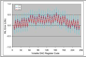
**FIGURE 2-57:** INL vs. Code (code = 6 to 250) and  $V_{DD}$  (2.7V, 5V, 5.5V) (**MCP4706**).  $V_{REF1}:V_{REF0} = 10, G = 1, V_{REF} = V_{DD}/2, Temp = +25°C.$
