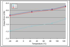
**FIGURE 2-84:** Output Error vs. Temperature (MCP4706).  $V_{DD}$  = 2.7V and 5V,  $V_{REF1}$ : $V_{REF0}$  = 10, G = 0,  $V_{REF}$  =  $V_{DD}$ , Code = 250.
