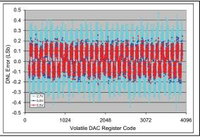
**FIGURE 2-58:** DNL vs. Code (code = 100 to 4000) and  $V_{DD}$  (2.7V, 5V, 5.5V) (**MCP4726**).  $V_{REF1}:V_{REF0} = 10, G = 1, V_{REF} = V_{DD}/2,$ Temp = +25°C.
