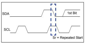
FIGURE 5-5: Repeat Start Condition Waveform.
