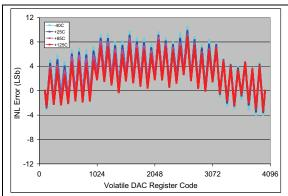
**FIGURE 2-4:** INL vs. Code (code = 100 to 4000) and Temperature (**MCP4726**).  $V_{DD} = 2.7V, V_{REF1}:V_{REF0} = 00.$
