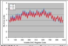
**FIGURE 2-2:** INL vs. Code (code = 25 to 1000) and Temperature (MCP4716).  $V_{DD} = 5V$ ,  $V_{REF1}$ : $V_{REF0} = 00$ .
