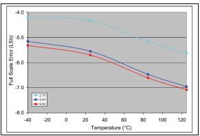
**FIGURE 2-35:** Full-Scale Error (FSE) vs. Temperature (MCP4716).  $V_{--} = 2 TV V_{--} = 10 C = 0$
