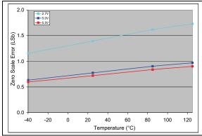
**FIGURE 2-31:** Zero-Scale Error (ZSE) vs. Temperature (**MCP4726**).
