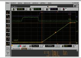
FIGURE 2-96: Full-Scale Settling Time (000h to FFFh) (MCP4726).
