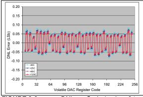
FIGURE 2-9:DNL vs. Code (code = 6 to250) and Temperature (MCP4706). $V_{DD}$  = 5V,  $V_{REF1}$ :  $V_{REF0}$  = 00.
