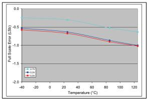
FIGURE 2-54:Full-Scale Error (FSE) vs.Temperature (MCP4706). $V_{DD}$  = 2.7V,  $V_{REF1}$ :  $V_{REF0}$  = 11, G = 0, $V_{REF}$  =  $V_{DD}$ .
