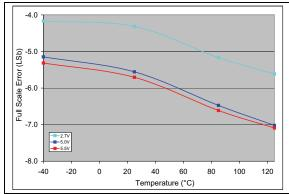
FIGURE 2-53:Full-Scale Error (FSE) vs.Temperature (MCP4716). $V_{DD} = 2.7V$ ,  $V_{REF1}$ :  $V_{REF0} = 11$ , G = 0, $V_{REF} = V_{DD}$ .
