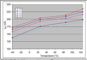
FIGURE 2-88: $I_{DD}$  vs. Temperature. $V_{DD}$  = 2.7V and 5V,  $V_{REF1}$ :  $V_{REF0}$  = 00.
