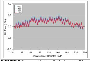
FIGURE 2-3:INL vs. Code (code = 6 to250) and Temperature (MCP4706). $V_{DD}$  = 5V,  $V_{REF1}$ :  $V_{REF0}$  = 00.
