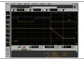
FIGURE 2-99: Half-Scale Settling Time (C00h to 400h) (MCP4726).
