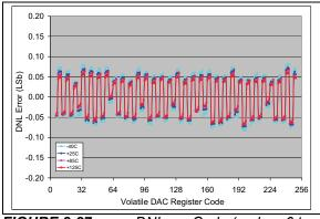
**FIGURE 2-27:** DNL vs. Code (code = 6 to 250) and Temperature (MCP4706).  $V_{DD} = 5V$ ,  $V_{REF1}$ :  $V_{REF0} = 10$ , G = 0,  $V_{REF} = V_{DD}$ .
