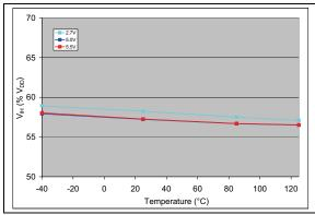
**FIGURE 2-92:** V<sub>IH</sub> Threshold of SDA/SCL Inputs vs. Temperature and V<sub>DD</sub>.
