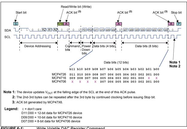
FIGURE 6-1: Write Volatile DAC Register Command.
