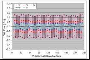
**FIGURE 2-72:** DNL vs. Code (code = 6 to 250) and  $V_{REF}$  (**MCP4706**).  $V_{DD} = 5V$ ,  $V_{REF1}$ :  $V_{REF0} = 10$ , G = 0,  $V_{RFF} = 1V$ , 2V, 3V, 4V, and 5V, Temp = +25°C.
