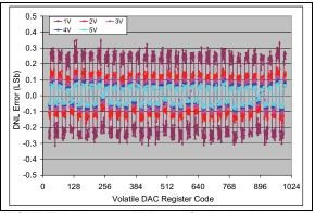
**FIGURE 2-71:** DNL vs. Code (code = 25 to 1000) and  $V_{REF}$  (MCP4716).  $V_{DD} = 5V$ ,  $V_{REF1}$ :  $V_{REF0} = 10$ , G = 0,
