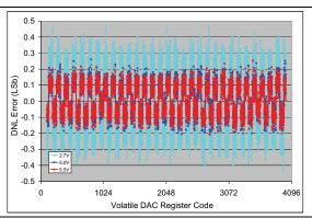
**FIGURE 2-64:** DNL vs. Code (code = 100 to 4000) and  $V_{DD}$  (2.7V, 5V, 5.5V) (**MCP4726**).  $V_{REF1}:V_{REF0} = 11$ , G = 1,  $V_{REF} = V_{DD}/2$ , Temp = +25°C.
