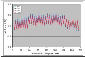
FIGURE 2-6:INL vs. Code (code = 6 to250) and Temperature (MCP4706). $V_{DD} = 2.7V, V_{REF1}: V_{REF0} = 00.$
