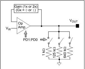
**FIGURE 4-5:** Op Amp to V<sub>OUT</sub> Pin Block Diagram.
