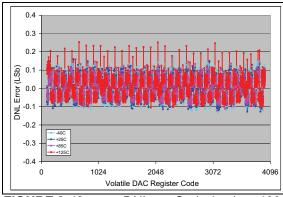
**FIGURE 2-43:** DNL vs. Code (code = 100 to 4000) and Temperature (**MCP4726**).  $V_{DD} = 5V$ ,  $V_{REF1}$ : $V_{REF0} = 11$ , G = 0,  $V_{REF} = V_{DD}$ .
