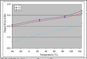
**FIGURE 2-86:** Output Error vs. Temperature (MCP4716).  $V_{DD} = 2.7V$  and 5V,  $V_{REF1}:V_{REF0} = 11$ , G = 0,  $V_{REF} = V_{DD}$ , Code = 1000.
