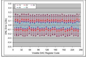
**FIGURE 2-78:** DNL vs. Code (code = 6 to 250) and  $V_{REF}$  (MCP4706).  $V_{DD} = 5V$ ,  $V_{REF1}$ : $V_{REF0} = 11$ , G = 0,  $V_{REF} = 1V$ , 2V, 3V, 4V, and 5V, Temp = +25°C.
