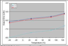
**FIGURE 2-80:** Output Error vs. Temperature (MCP4716).  $V_{DD}$  = 2.7V and 5V,  $V_{REF1}$ :  $V_{REF0}$  = 00, Code = 1000.
