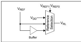
**FIGURE 4-2:** Resistor Ladder Reference Voltage Selection Block Diagram.
