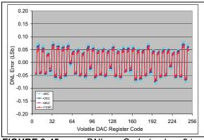
FIGURE 2-45:DNL vs. Code (code = 6 to250) and Temperature (MCP4706). $V_{DD} = 5V$ ,  $V_{REF1}$ :  $V_{REF0} = 11$ , G = 0, $V_{REF} = V_{DD}$ .
