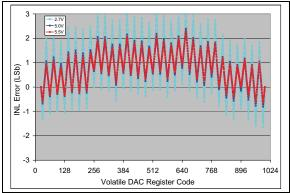
**FIGURE 2-62:** INL vs. Code (code = 25 to 1000) and  $V_{DD}$  (2.7V, 5V, 5.5V) (**MCP4716**).  $V_{REF1}:V_{REF0} = 11$ , G = 1,  $V_{REF} = V_{DD}/2$ , Temp = +25°C.
