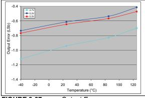
**FIGURE 2-87:** Output Error vs. Temperature (MCP4706).  $V_{DD} = 2.7V$  and 5V,  $V_{REF1}:V_{REF0} = 11$ , G = 0,  $V_{REF} = V_{DD}$ , Code = 250.
