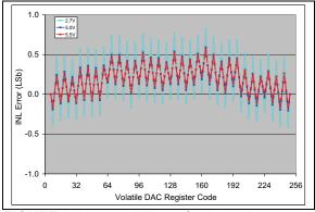
**FIGURE 2-63:** INL vs. Code (code = 6 to 250) and  $V_{DD}$  (2.7V, 5V, 5.5V) (**MCP4706**).  $V_{REF1}:V_{REF0} = 11$ , G = 1,  $V_{REF} = V_{DD}/2$ , Temp = +25°C.
