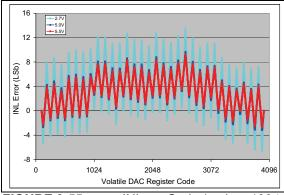
**FIGURE 2-55:** INL vs. Code (code = 100 to 4000) and  $V_{DD}$  (2.7V, 5V, 5.5V) (**MCP4726**).  $V_{REF1}:V_{REF0} = 10, G = 1, V_{REF} = V_{DD}/2,$ Temp = +25°C.
