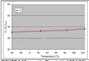
**FIGURE 2-93:** V<sub>IL</sub> Threshold of SDA/SCL Inputs vs. Temperature and V<sub>DD</sub>.
