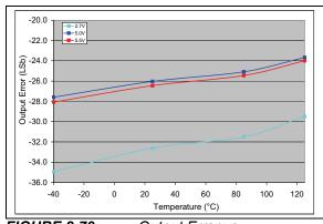
**FIGURE 2-79:** Output Error vs. Temperature (**MCP4726**).  $V_{DD}$  = 2.7V and 5V,  $V_{REF1}$ :  $V_{REF0}$  = 00, Code = 4000.
