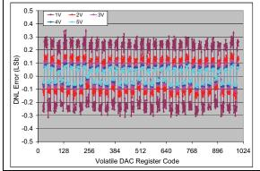
FIGURE 2-77: DNL vs. Code (code = 25 to 1000) and  $V_{REF}$  (MCP4716).  $V_{DD} = 5V$ ,  $V_{REF1}$ :  $V_{REF0} = 11$ , G = 0,  $V_{REF} = 1V$ , 2V, 3V, 4V, and 5V, Temp = +25°C.
