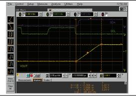
FIGURE 2-98: Half-Scale Settling Time (400h to C00h) (MCP4726).
