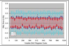
**FIGURE 2-59:** DNL vs. Code (code = 25 to 1000) and  $V_{DD}$  (2.7V, 5V, 5.5V) (**MCP4716**).  $V_{REF1}:V_{REF0} = 10, G = 1, V_{REF} = V_{DD}/2,$ Temp = +25°C.
