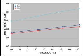
FIGURE 2-50:Zero-Scale Error (ZSE) vs.Temperature (MCP4716). $V_{DD} = 5V$ ,  $V_{REF1}$ :  $V_{REF0} = 11$ , G = 0, $V_{REF} = V_{DD}$ .
