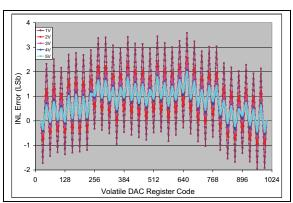
**FIGURE 2-74:** INL vs. Code (code = 25 to 1000) and  $V_{REF}$  (MCP4716).  $V_{DD} = 5V$ ,  $V_{REF1}$ :  $V_{REF0} = 11$ , G = 0,  $V_{RFF} = 1V$ , 2V, 3V, 4V, and 5V, Temp = +25°C.
