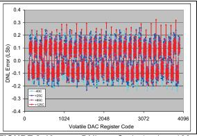
**FIGURE 2-10:** DNL vs. Code (code = 100 to 4000) and Temperature (**MCP4726**).  $V_{DD} = 2.7V, V_{REF1}: V_{REF0} = 00.$
