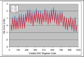
**FIGURE 2-5:** INL vs. Code (code = 25 to 1000) and Temperature (MCP4716). V<sub>DD</sub> = 2.7V, V<sub>REF1</sub>:V<sub>REF0</sub> = 00.
