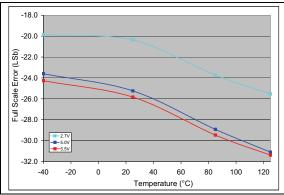
**FIGURE 2-52:** Full-Scale Error (FSE) vs. Temperature (**MCP4726**).  $V_{PD} = 2.7V$ ,  $V_{PDD} = 11$ , G = 0
