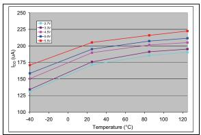
FIGURE 2-90: $I_{DD}$  vs. Temperature. $V_{DD}$  = 2.7V and 5V,  $V_{REF1}$ :  $V_{REF0}$  = 11, G = 0, $V_{REF}$  =  $V_{DD}$ .
