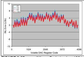
**FIGURE 2-37:** INL vs. Code (code = 100 to 4000) and Temperature (**MCP4726**). V<sub>DD</sub> = 5V, V<sub>REF1</sub>:V<sub>REF0</sub> = 11, G = 0,
