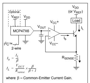
FIGURE 8-8: Digitally-Controlled Current Source.
