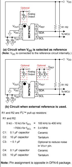
**FIGURE 8-2:** Example MCP47X6 Circuit with SOT-23 package.
