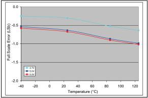
**FIGURE 2-36:** Full-Scale Error (FSE) vs. Temperature (MCP4706).  $V_{DD} = 2.7V, V_{REF1}: V_{REF0} = 10, G = 0,$  $V_{REF} = V_{DD}.$
