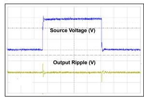
**FIGURE 2-17:** Line Transient Response  $(I_{LOAD} = 10 \text{ mA}) (100 \text{ µs/Div}).$
