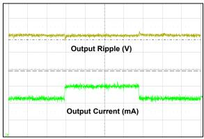
**FIGURE 2-14:** Load Transient Response  $(I_{LOAD} = 50 \text{ mA/Div}, \text{ Output: } 100 \text{ mV/Div}, \text{ Time: } 100 \text{ µs/Div}).$
