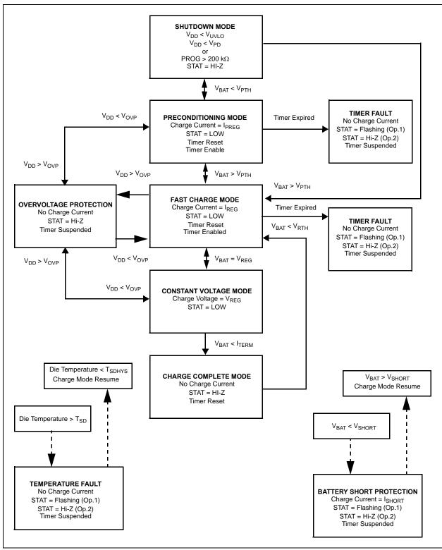
FIGURE 4-1: The MCP73213 Flow Chart.
