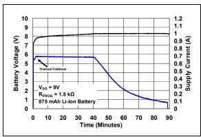
**FIGURE 6-2:** Typical Charge Profile (875 mAh Li-Ion Battery).
