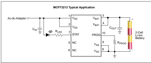
FIGURE 6-1: Typical Application Circuit.
