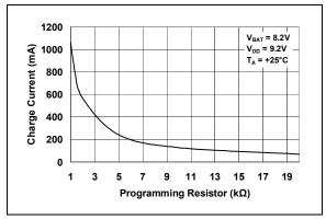
**FIGURE 2-5:** Charge Current ( $I_{OUT}$ ) vs. Programming Resistor ( $R_{PROG}$ ).
