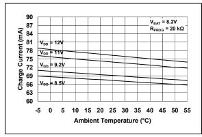
**FIGURE 2-9:** Charge Current ( $I_{OUT}$ ) vs. Ambient Temperature ( $T_A$ ).
