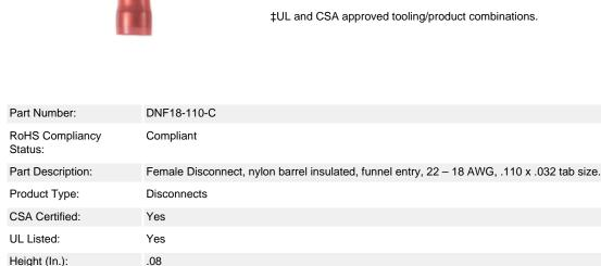
Height (In.): .08 Length (In.): .69 Width (In.): .15 Max. Ins.: .100 Panduit Color Code: Red Tab Size (In.): .110 x .032 CT-600-A‡, CT-1525‡, CT-2500‡ Tool: Wire Range: 22 - 18 AWG Min. Order UOM: PC
