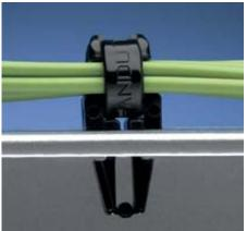
• Push mounts require no adhesive backing or additional mounting hardware. They are inserted into pre-drilled holes. Can be used where only one side of the panel is accessible. This push mount does not have tensioning wings.
