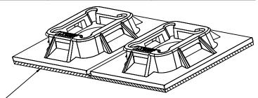
ADHESIVE BACKING: RUBBER BASED ADHESIVE PRESSURE
