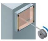
Note: When the floating blanking function is used, the size of the min. sensing object is changed. Refer to "**PRECAUTIONS** FOR PROPER USE" (p.36) for details.
