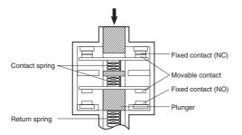
Conforms to EN60947-5-1 Direct Opening Operation ←
