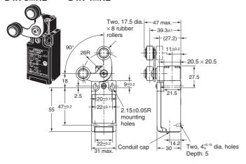
**Fork Lever Lock** (Left Operation) D4N-1☐LE D4N-2□LE D4N-3□LE D4N-4□LE -47 max -39.3±1 → Two, 17.5 dia. × (27.2) 8 rubber rollers  $20.5 \times 20.5$ 2.15±0.05R mounting holes Two, 4<sup>+0</sup> dia. holes Conduit cap Depth: 5
