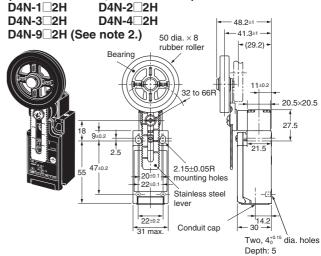
Note: 1. Unless otherwise specified, a tolerance of  $\pm 0.4$  mm applies to all dimensions.
