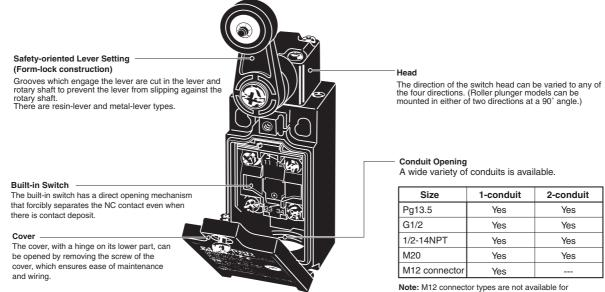
Note: M12 connector types are not available fo Switches with three contacts.
