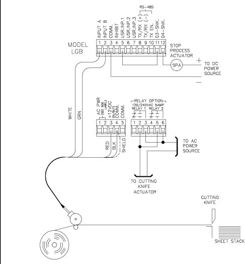
Preset value  $P_1$  (*Process count*) is programmed for the first length to be cut for the order and Preset value  $P_2$  (*Process count*) for the second length.
