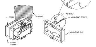
farthest forward slot possible. To achieve a proper seal, tighten the latch screws evenly until the unit is snug in the panel (Torque to approx. 28 to 36 in-oz [0.202 to 0.26 N-m]). Do not over-tighten the screws.
