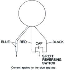
leads produces CW rotation. Switching the current to the blue and black leads produces CCW rotation.
