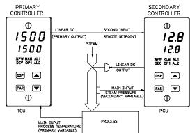
Similar to internal cascade control, external cascade control differs by the employment of two controllers, one of which is equipped with a second analog input configured as a remote setpoint. A PCU controls the secondary loop, while a TCU controls the primary loop.
