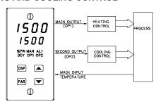
The TCU has dual outputs for providing heating and cooling to those processes that require them. Many extruder applications require both heating and cooling to maintain accurate extruder barrel and die temperatures. The TCU is easily configured for these applications.
