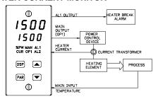
The Heater Current Monitor serves as a heater element fail sentry, so operators can take corrective action before significant process errors occur in the event of a failure. The actual heater current can be viewed in the secondary display and/or a heater break alarm output can be programmed.
