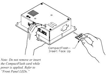
Information stored on a CompactFlash card by a G306A can be read by a card reader attached to a PC. This information is stored in IBM (Windows®) PC compatible FAT16 file format.
